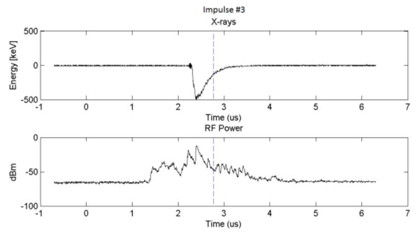
X-rays and RF power at 2.4 GHz for negative voltage impulse. Plot corresponds to a voltage impulse of -775 kV. Vertical dashed line indicates the breakdown time (Montanyà, et. al. 2014).
